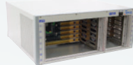
GX7110 3U/6U, 14-slot PXI chassis for use with a PXI Bus Expander
