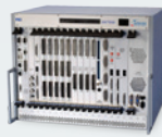
GX7010 6U, 20-Slot PXI chassis for use with a PXI Bus Expander
