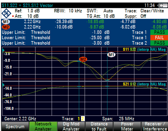
Vector network analyzer mode: For cable loss and antenna testing and characterization as well as distance to fault measurements. Two-port capability for transmission measurements
