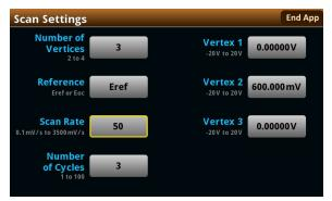
2450-EC Cyclic Voltammetry Test Configuration Screen
