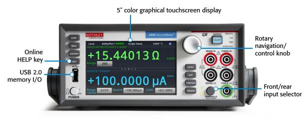
2450-EC front panel with high-resolution, capacitive touchscreen.
