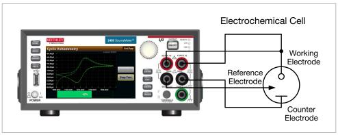
The 2450-EC can be easily connected to a 3-electrode cell.
