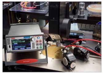
Characterize transistors with multiple SMU instruments on wafer or packaged transistors
