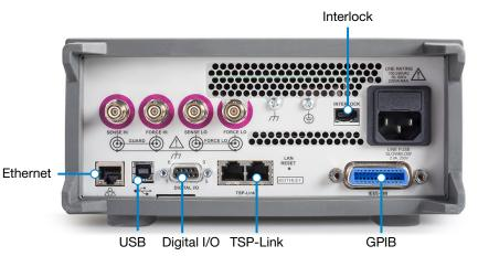
Rear panel connections are optimized for signal integrity and speed system setup.
