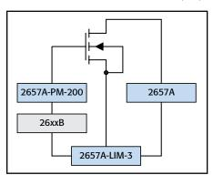
The Model 2657A can be combined with Series 2600B and Model 4200-SCS SMU instruments to support multi-terminal test capability. The Models 2657A-PM-200 Protection Module and 2657A-LIM-3 Low Interconnect Module make it easier to connect multiple instruments to a probe station safely (not required for connecting to the Model 8010 High Power Device Test Fixture).
