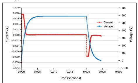
The dual high speed A/D converters sample as fast as 1µs per point, enabling full simultaneous characterization of both voltage and current.
