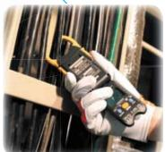
Sometimes it's easier to clamp the target wire at an angle.
