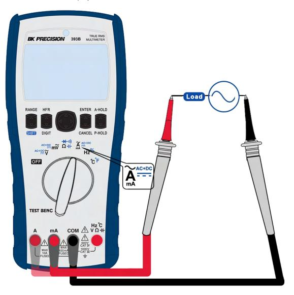
Figure 2.8 Current Measurement
