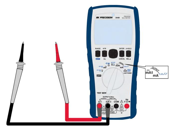
Figure 4.2 Source Mode Connection
