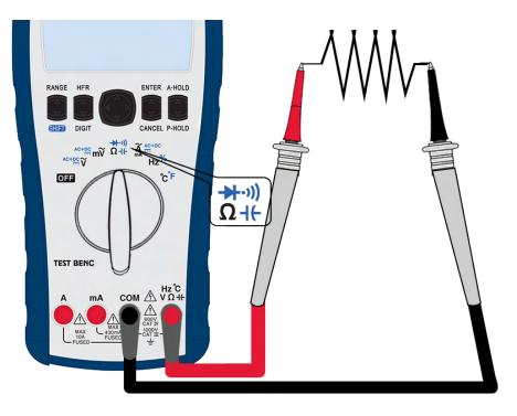
Figure 2.5 Resistance Measurement
