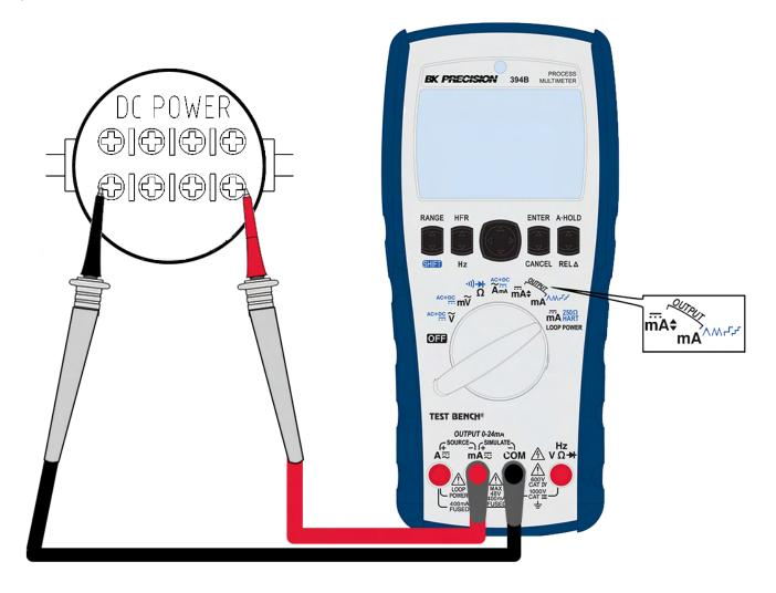
Figure 4.4 Loop Power Mode Connection
