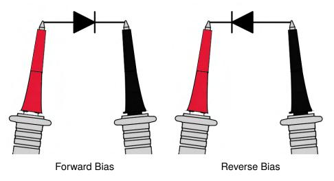
Figure 2.6 Testing Diodes
