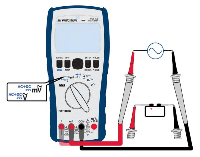
Figure 2.1 Voltage Measurement
