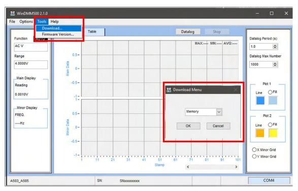
Figure 3.4 Import measurements with software
