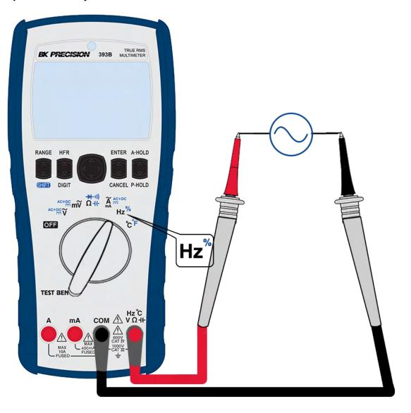
Figure 2.9 Frequency Measurement
