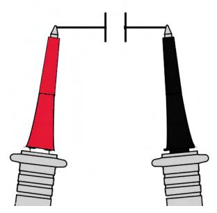
Figure 2.7 Capacitance Measurement
