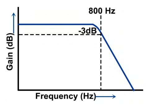
Figure 2.2 High Frequency Reject
