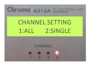
4. The Response setting may need to be set to insure the LED driver and LED Load does not oscillate. Chroma offers 5 settings for the Load response time ranging from 3kHz to 30Khz. The default setting is 3, or you can select the SET option and set the response from 1-5. With 1 being 3Khz and 5 being 30Khz bandwidth.
