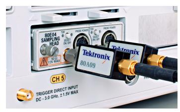
Sampling modules with dual electrical channels, such as the 80E04 dualchannel 20 GHz electrical sampling module with TDR, require two 80A09 devices. Step generators within the 80E04 TDR modules uses ≤ 250 mV. which is less than the diode threshold of the 80A09 device.
