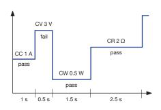
Up to 100 different sequences can be linked to run steps of various operating modes and loading conditions. Each step can be programmed with upper and lower pass/fail limits.
