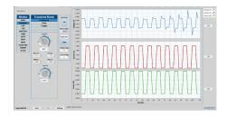
PC software is provided for generating and executing test sequences and measurement data logging without the need to write source code.
