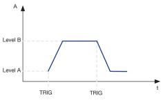
The DC load current will toggle between Level-A and Level-B following receipt of a trigger signal.
