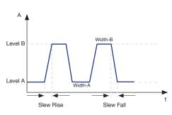
Switch continuously between A and B load current levels where rise/fall slew rates and level width can be adjusted.
