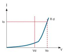
Figure - LED I-V Curve
