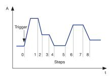
Each list mode program contains up to 100 user programmable steps. Save up to 10 list mode program files directly to internal memory for quick recall. Step parameters include current limit, step duration, and slew rate. This series supports extended list mode features with the ability to advance list steps upon receipt of an internal/external trigger. List mode programs can be configured and run from the front panel or remotely using the provided application software.
