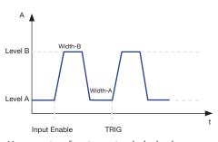
Upon receipt of a trigger signal, the load executes one pulse cycle then returns to load current level A.
