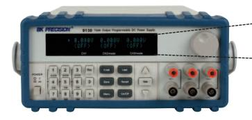
The 9130 is a fully programmable triple Output DC Power Supply delivering 0-30V/0-3A on 2 outputs and 0-5V/0-3A on 1 output. Each output is fully floating and outputs can be adjusted independently or connected in series or parallel to produce higher voltages or currents. The 9130 is ideally suited for applications in Electronic Test, Production and Service where multiple independent DC supplies are required and bench space is at a premium.
