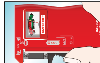
Testing 1.5 V battery (AAA, AA, C, D)
