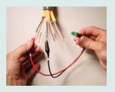
GREEN LED means wiring is properly identified.
