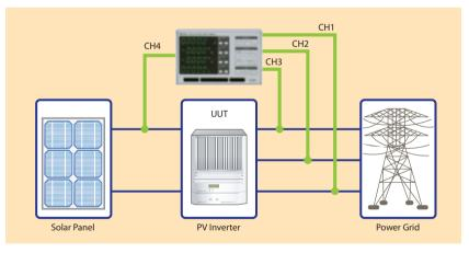
User could implement 3P3W (Three Phase Three Wire) wiring mode for three phase power measurement application. Such as AC motor inverter testing.
