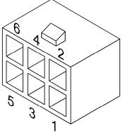
Two connectors are provided; pinouts are identical.
