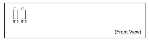
Figure 5-2. Display PWA Location of Potentiometers
