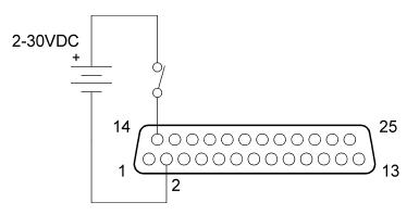
Figure 4-9. EXTERNAL–OFF with Voltage Source
