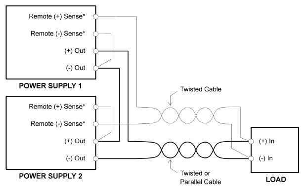
\*SETUP Switch Position-1, REM SNS, Set to ON
