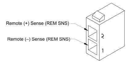
Figure 2-4. Remote Sense Connector
