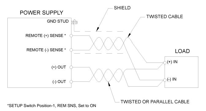
Figure 2-6. Single Load Connection with Remote Sensing
