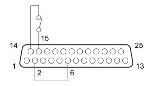
Figure 4-10. EXTERNAL–OFF with AUXILIARY 5 VDC OUTPUT
