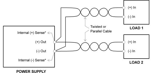
\* SETUP Switch Position-1, REM SNS, Set to OFF
