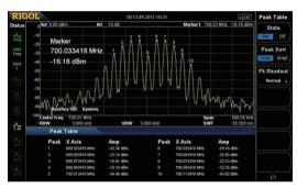
Phase noise < -98 dBc/Hz @10 kHz offset (DSA832/875)
