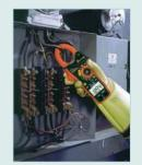
CAT IV -600V safety rating for added protection and True RMS feature gives you accurate readings of non-sinusoidal waveforms.
