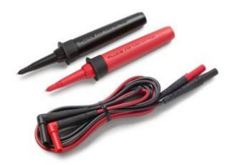
SureGrip Fused Test Probe and Test Lead set with built-in replaceable fuses for additional measurement protection. If the probe fuse does blow, these fused test probes will still allow the meter to indicate live voltage, helping to prevent a possible misreading of no voltage present. These modular probes ship with the Fluke TL224 silicone test leads. Rated to CAT III 1000 V, these probes have removable tip guards for reduced probe tip exposure.
