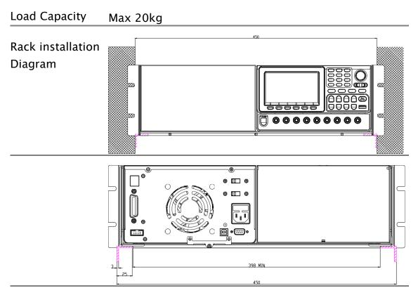
Note The minimum width that is needed to be supported on the L-brackets.
