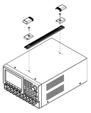
2. Remove the foot pads from the GPP power supply.
