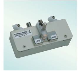
SMD TEST FIXTURE 9699 Electrodes on bottom for SMD DC to 120 MHz Test sample dimensions: 1.0mm (0.04in) to 4.0mm (0.16in) wide, maximum 1.5mm (0.06in) high
