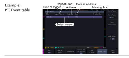
Example: I<sup>2</sup>C Data Detail Time of trigger Address Cont Table
