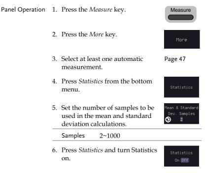
7. The statistics for each automatic measurement will appear at the bottom of the display in a table.
