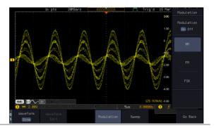
Panel Operation 1. Select the carrier waveform from the GEN1 Setup/GEN2 Setup menu:
