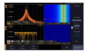
5. Press the *Run/Stop* key followed by pressing the *Slice* key and rotate the *VARIABLE* knob to observe input signal. And it's spectrogram on the same date time axis.
