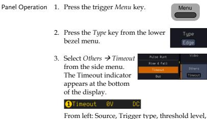
From left: Source, Trigger type, threshold leve coupling 4. Press *Source* from the lower menu.
