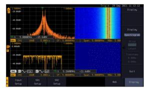
3. Choose a display mode by toggling between *Spectrum* button and *Spectrogram* button using the *VARIABLE* knob.
