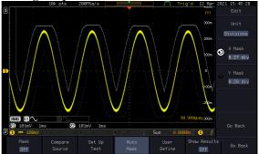
7. Press the *Y Mask* button from the side menu and use the *VARIABLE* knob to adjust the vertical deviation of the mask compared to its original pattern.
