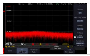
FFT-split The time domain waveform is shown in the upper section, whereas the FFT display is shown in the lower section.
