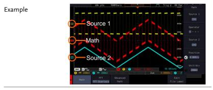
Position and Unit To move the math waveform vertically, press the *Position* key from **O B**. **BODI** the side menu and use the VARIABLE knob to set the position.
