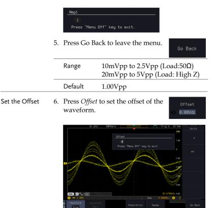
7. Use the Left and Right arrow keys to select a base unit and use VARIABLE knob to increase the offset by that base unit, as shown in the Offset window. Or use the numerical keypad to input value.
