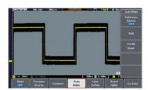
The MSO-2000E series provides the Mask function, which allows users to apply Auto Mask and user-defined Mask to determine whether the quality of the product meets the regulation. Via user-defined mask, users can set up to 8 areas and each area is up to
