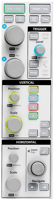
Efficient and intuitive front panel provides critical controls while still leaving room for the massive 15.6" high definition display.
