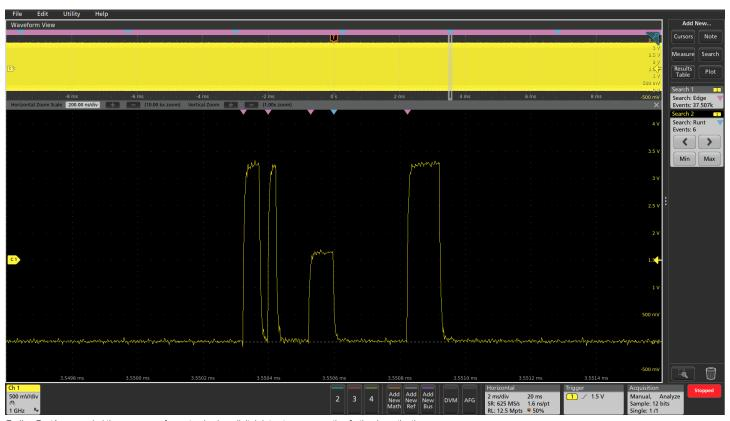
Earlier, FastAcg revealed the presence of a runt pulse in a digital data stream prompting further investigation.
