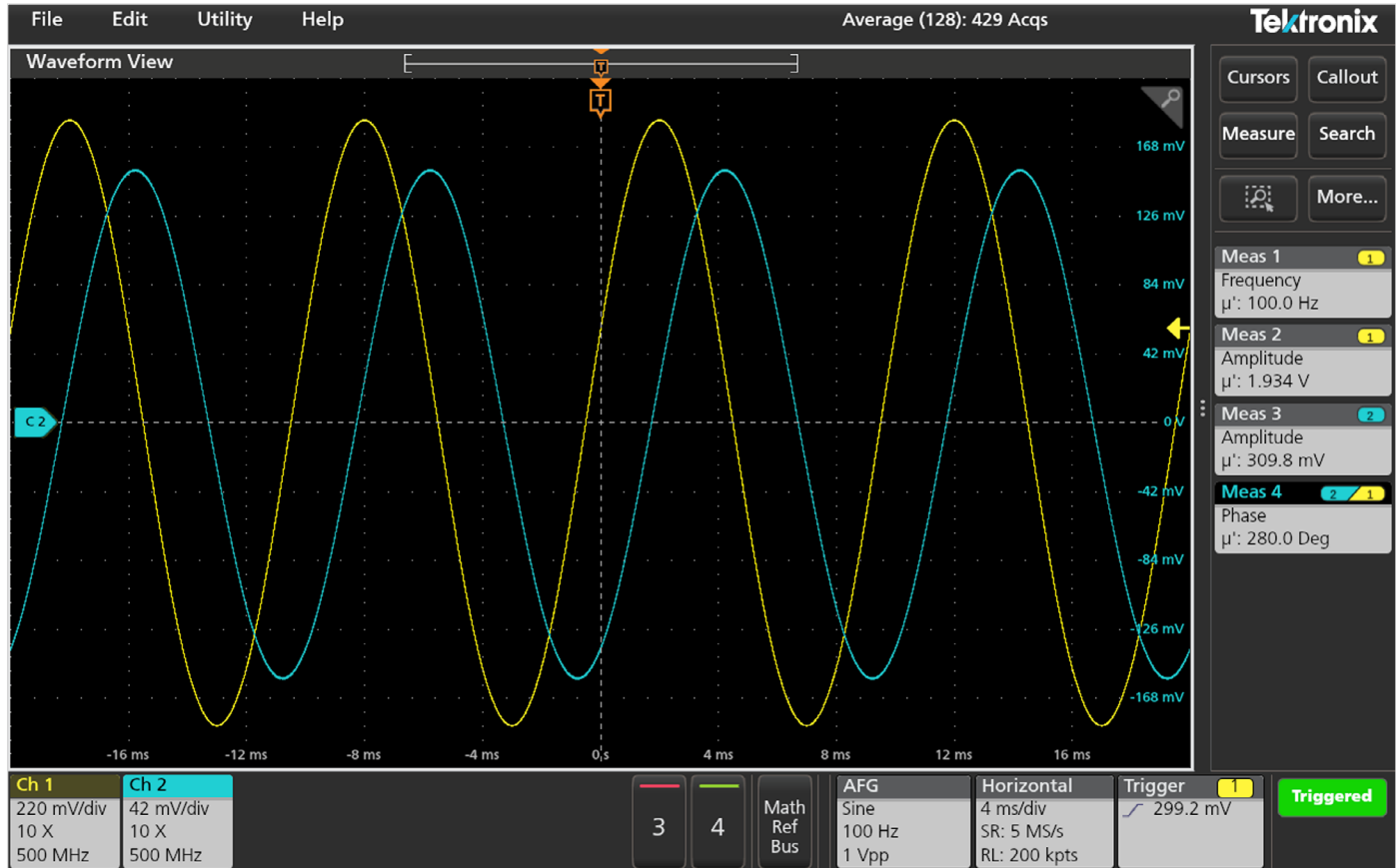
Figure 4. Voltage waveforms and measurements taken at nodes A1 and A2.
