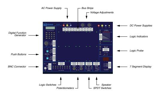
Figure 1 PB-505A Components
