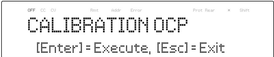
3. Press **Enter** to run the OCP calibration or press **Esc** to abort. The OCP calibration is an automatic process that will take about 20 to 30 seconds.
