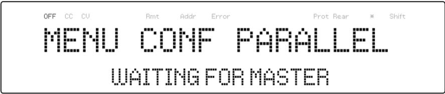
If the master unit has found the slave unit, the slave unit will be controlled by the master unit and the following will be displayed:
