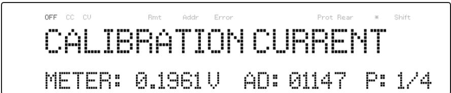
The *P: 1/4* signifies there are 4 points to be calibrated, and the current calibration point is 1.
