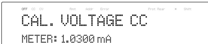
3. Input the current reading from the DMM into the **METER** parameter by using the numeric keypad and press **Enter**.
