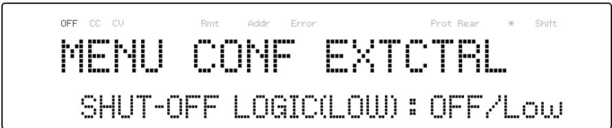
4. Use the rotary knob to select the setting of **OFF/Low** (Falling Edge) or **ON/Low** (Rising Edge) and press **Enter**.
