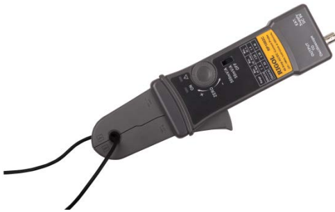
Figure 2 Connection between the Test Clamp and Conductor
