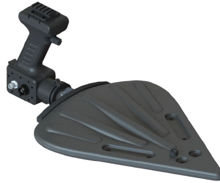
Alaris direction-finding smart antenna.
