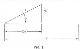
the reference voltage divider. The phase shift is an angle whose tangent is equal to Mo/EX. For angles less than 6 deg, multiply the ratio Mo/EX by 57.3 deg to calculate a
