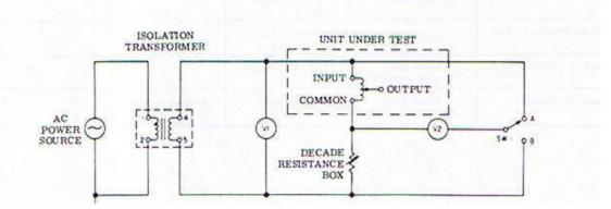
Figure 5-1. Impedance Test Setup
