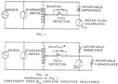
Since we can make the ratio transformer operate essentially unloaded by this method, meters with impedance as low as desired can be calibrated with no loss in accuracy.
