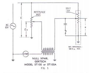
phase angle within the accuracy of the measurement technique. If a constant reference source is used, the dial of the voltmeter can be calibrated in phase shift directly.
