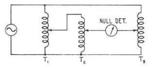
$(R_1 + E_1) (R_2 + E_2) = (R_3 + E_3)$  at Balance if we choose  $R_1 = R_2 = .5$
