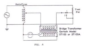
The circuit shown in Fig. A is a variation on the method described in the preceding article. Leads may be changed instead of using a switch.
