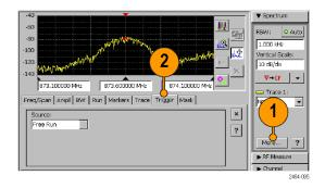
Tap the Source field and select the trigger type. The External setting requires a TTL-level trigger signal at the Trigger/Timing connector.
