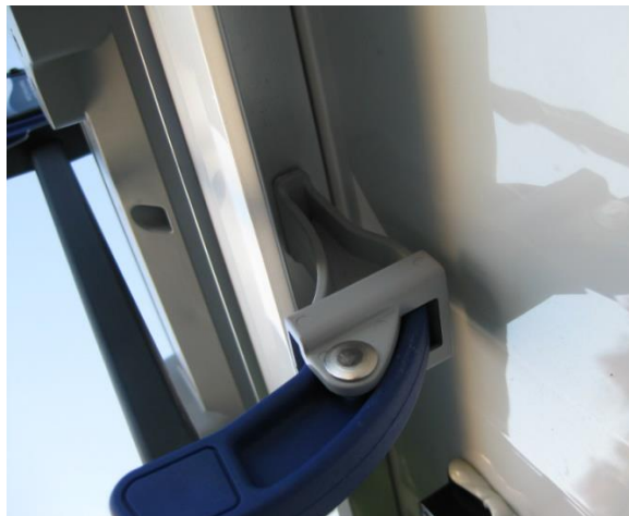
Figure 23. Tip of frame clamp properly seated on inside surface of module frame
