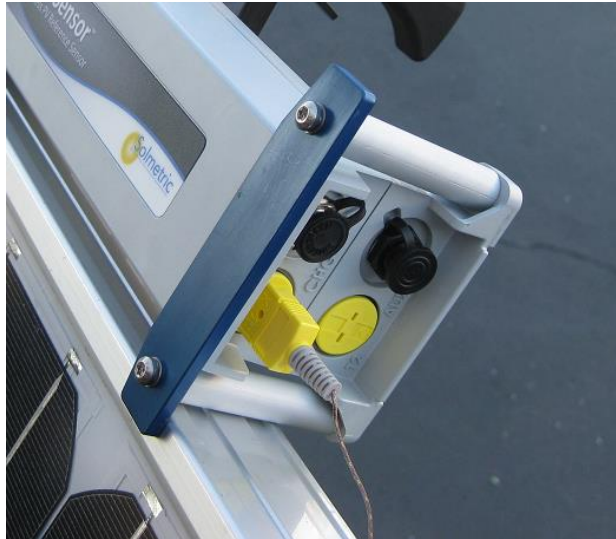
Figure 24. Thermocouple plugged into the TC1 connector.
