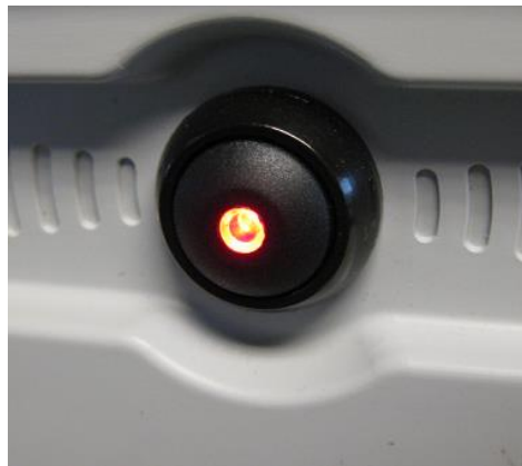
Figure 26. SolSensor pushbutton with LED lit. LED blinks until wireless network is established, after which it remains on.
