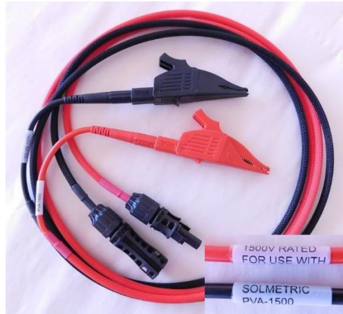
Figure 1. Test leads and clips rated for use with the PVA-1500xx
