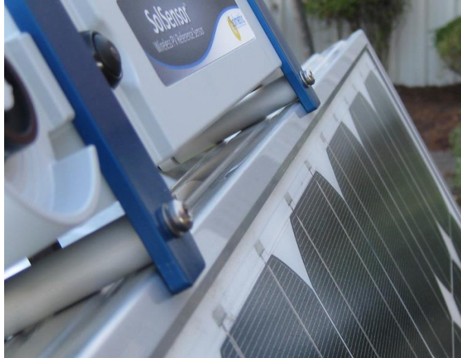
Figure 22. SolSensor correctly seated along the upper horizontal leg of the module frame.
