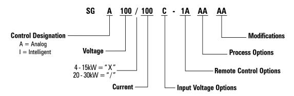
(For units up to 999A, Current is represented in numeric format (rounded to whole Amp), e.g., above "100" represents 100A. For units at 1000A and above, the current is represented by the format "XKX", e.g., 1K2 represents 1200A)
