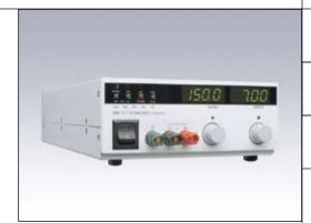
The XHR is power factor corrected for low current draw - only 11 amps at 120 volts AC for 1000 watts - and reduced generation of input current harmonics. Zero voltage or "soft switching" virtually eliminates switching transients for high efficiency, low noise and high reliability. It is also stackable, with a small footprint, front panel binding post connectors, and a low current requirement with universal input, making the XHR ideal for benchtop applications.
