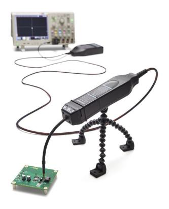
The Tektronix TIVM and TIVH Series IsoVu<sup>™</sup> Measurement Systems offer galvanically isolated measurement solutions for accurately resolving high bandwidth, differential signals up to ±2500 V in the presence of large common mode voltages with the best in class common mode rejection performance across its bandwidth.
