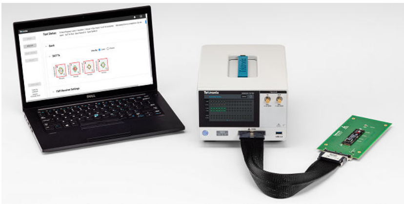
Figure 19: Setup using M.2 Slot adapter for SSD testing.
