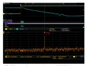
4. The PLL eventually settles on the correct 2.400 GHz frequency about 320 μs after the VCO was enabled.
