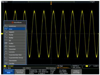
Waveform type selection in the integrated AFG.
