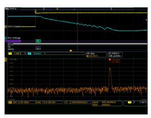
2. Spectrum Time is moved about 90 µs to the right. At this point, the spectrum shows that the PLL is in the process of tuning to the correct frequency (2.400 GHz). It has made it down to 2.4924 GHz.
