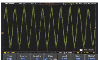
Unfiltered Waveform with Noise Interference
