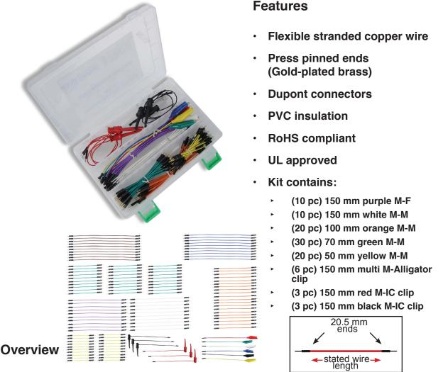
The WK-6 Wire Jumper Kit contains 112 pre-cut #24 gauge insulated stranded wire. Each wire comes with gold-plated brass pressed pins on each end to allow for extended insertion life and maximum surface contact. This kit also contains 10 male to female, 6 male to alligator clip, and 6 male to IC clip jumper wires. The WK-6 comes in a convenient plastic case and comes with both UL and RoHS.
