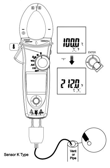
Don't take any high voltage measurement prior to accurate °C/°F measurements.
