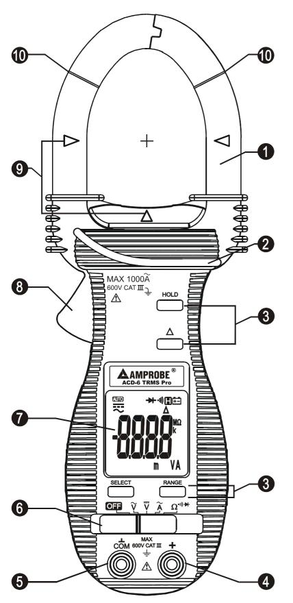
1) Transformer Clamp Jaw for AC current magnetic field pick up
