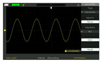
Figure 3.49 – Save Waveform Screen (To Internal Storage)
