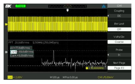
Figure 3.15 – Measuring FFT Amplitude
