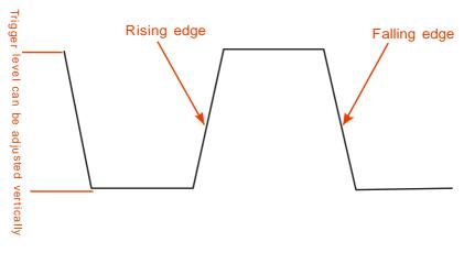
Figure 3.28 – Rising and Falling Edge Illustration
