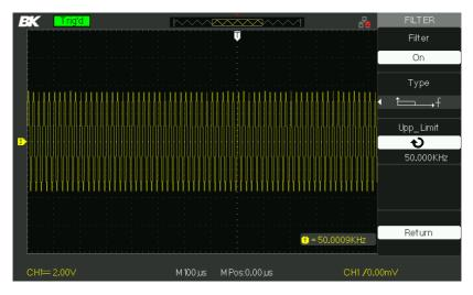
Figure 3.12 – Digital Filter Adjustment Screen
