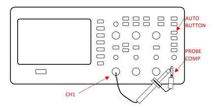
Figure 2.6 – Probe Compensation Setup
