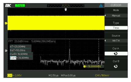
Figure 3.16 – Measuring FFT Frequency
