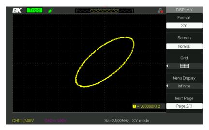
Figure 4.4 – Out of Phase Signals in XY Mode (45 degrees)
