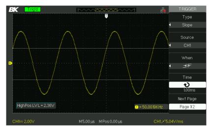
Figure 3.25 – Slope Trigger Menu 1
