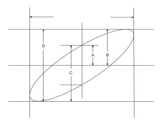
Figure 4.3 - Out of Phase Signals (45 degrees)
