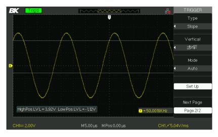
Figure 3.26 – Slope Trigger Menu 2
