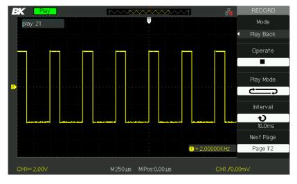
Figure 3.68 – Playback Menu Screen 1 (Recode Mode)
