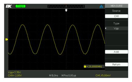
Figure 3.41 – Measuring Vpp Parameters
