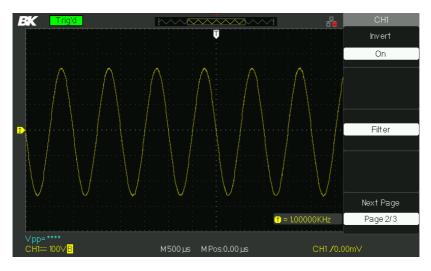
Figure 3.10 – Invert Waveform Screen
