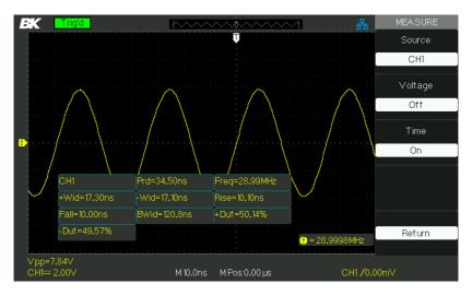
Figure 3.42 – Measuring All Time Parameters
