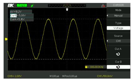
Figure 4.2 – Taking Cursor Measurements (Voltage)
