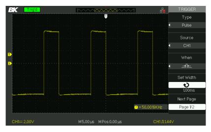
Figure 3.22 – Pulse Trigger Menu 1
