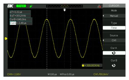
Figure 4.1 – Taking Cursor Measurements (Time)
