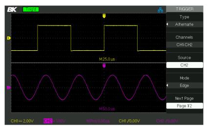
Figure 3.27 – Alternate Trigger Menu
