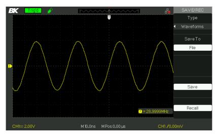
Figure 3.50– Save Waveform Screen (To Flash Drive)
