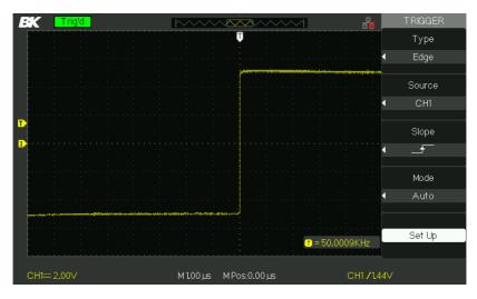
Figure 3.21 – Trigger Menu Screen
