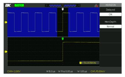
3. Press the "Delayed" option button to select "On".
