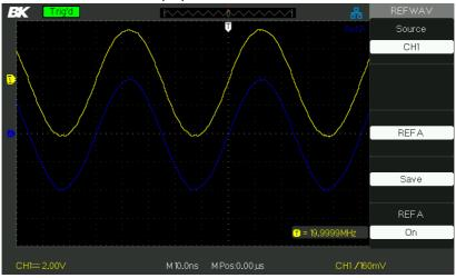
Press the Ref button to display the "Reference waveform menu".
