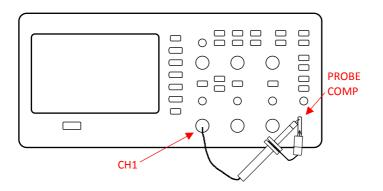
Figure 2.3 – Probe Compensation
