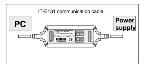
**Note:** It is **not possible** to connect the DB9 TTL connector on the power supply's rear panel supply via a <u>standard</u> RS232 cable to a PC's RS232 port.
