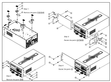
Figure 13- 3U Single Supply Rackmount Installation
