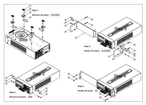
Figure 11- 2U Single Supply Rackmount Installation
