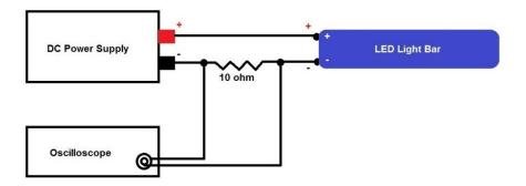
Figure 20- LED Testing Example
