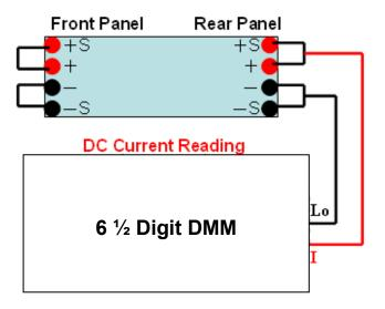
Figure 31 - Current Calibration Setup
