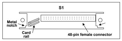
3. The interface card should go right below the metal notches on both sides and fit in between the inner card rails, also on both sides. Slide the card down carefully. When it touches the 48-pin connector, slowly push the card all the way in until the panel of the interface card aligns with the rear panel of the power supply.
