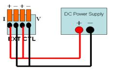
Figure 36- Single Channel Analog Control Calibration Setup
