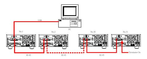
Figure 15- RS-485 Setup to Control Multiple Supplies (USB)
