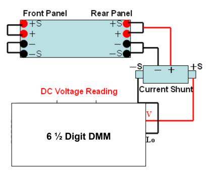
Figure 32- Current Calibration with Shunt
