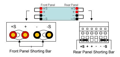
Figure 16-Local Sense with Shorting Bar
