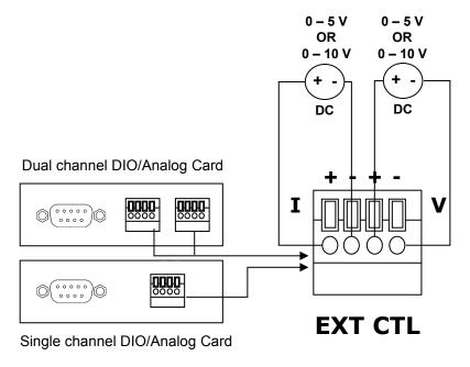
Figure 23- External Voltage Control
