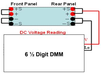
Figure 33- Voltage Calibration Setup
