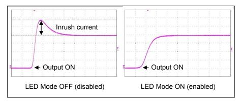
Figure 21 - Inrush Current With and Without LED Mode Enabled
