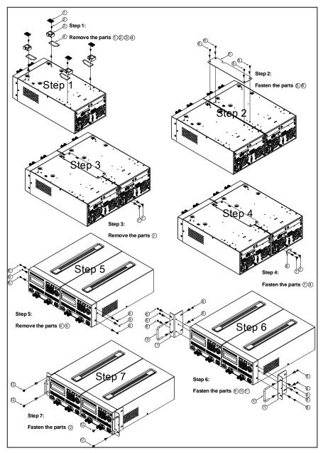
Figure 14–3U Dual Supplies Rackmount Installation
