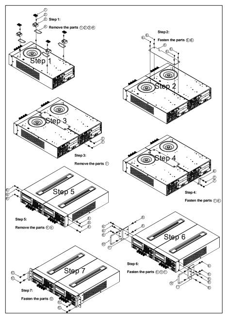
Figure 12- 2U Dual Supplies Rackmount Installation
