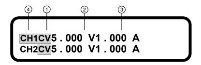
Figure 10- Dual Channel Main Display
