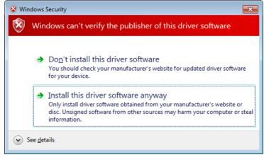
12. The driver will now install. Once finished, under "Device Manager", you should see under "Ports (COM & LPT)" an item labeled "BK Precision USB to Serial Converter (COM#)". The "COM#" is the com port that can be used to access the virtual COM port for remote communication.
