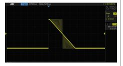
Sharp rise/fall times can be set from 8.4 ns up to 22.4 s with adjustment steps as small as 100 ps.
