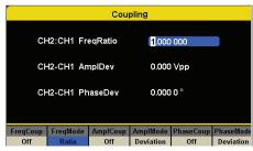
Customize channel coupling using frequency, amplitude, and phase. Enable automatic tracking between channels using deviation or ratio.
