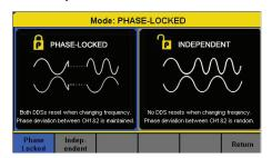
Phase-lock maintains phase deviation over both channels. In independent mode, the phase deviation between CHI and CH2 changes at random allowing for smoother frequency transitions.
