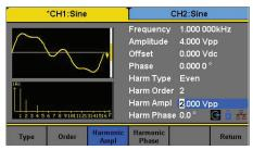
Quickly output harmonics up to the l6th order with independent amplitude and phase settings.
