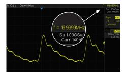
Built-in arbitrary waveform at 20 MHz, 300 MSa/s
