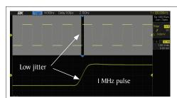
This series is equipped with advanced digital signal processing to reduce jitter and produce clean pulse waveforms.
