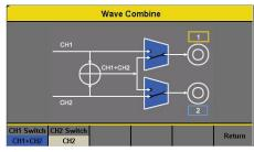
Create complex waveforms by internally adding each channel's waveform and outputting the combined waveform on channel I or 2.
