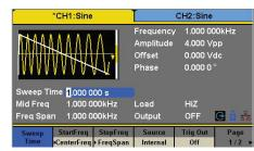
Perform linear or log sweep functions with up or down directional control. The sweep source can be set to internal, external, or manual.
