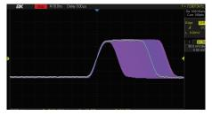
The pulse width is adjustable to a minimum of 16.3 ns. Shown above is the oscilloscope view of the pulse width being incremented using the generators rotary control knob.
