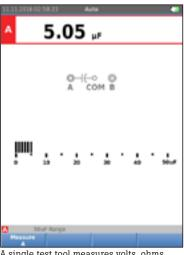
A single test tool measures volts, ohms, amps or capacitance, in addition to displaying waveforms.
