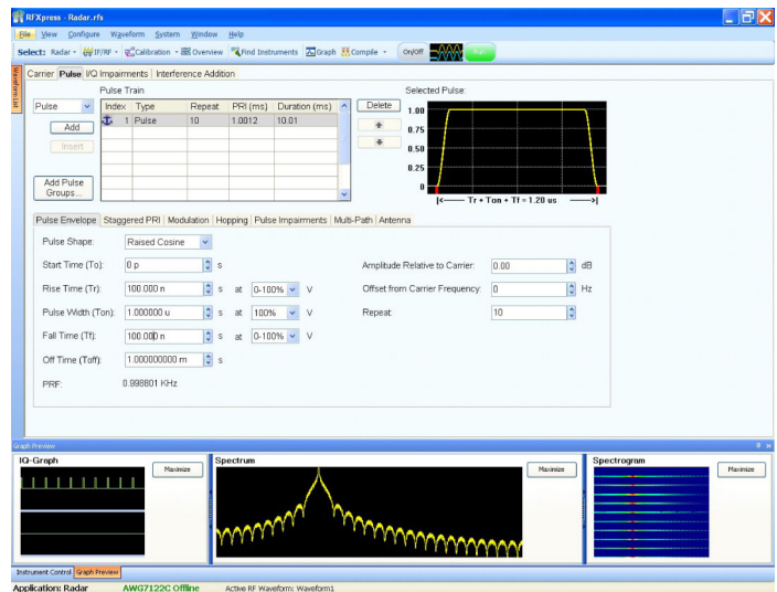
AWG radar pulses created with AWG70000A and RFXpress.
