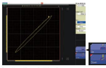
Pen up/down while recording X-Y waveforms
