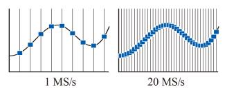
High-speed sampling allows you to measure the rising edge of pulses and detect anomaly operations and instantaneous waveforms that occur suddenly with high precision.
