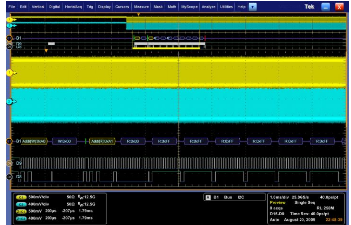
10 ms duration capture of synchronous high-speed and low-speed signals at 25 GS/s.
