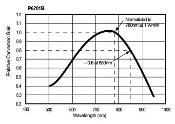
Figure 3: P6701B typical wavelength dependent gain (25 °C)
